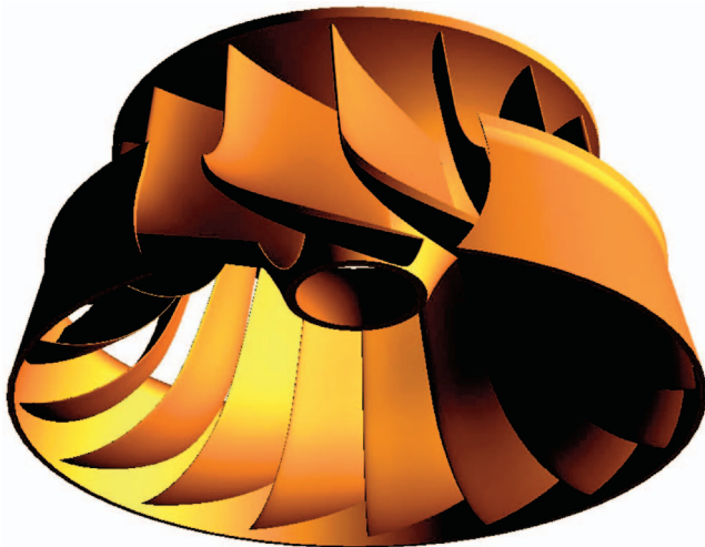
Fig. 16 Configuration of new runner design
